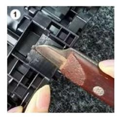
Take a knife and flatten the surface for the chip holder.
