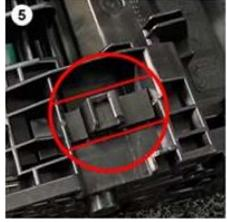
Stick the chip holder in the original position as it was before. This must be done with care to align properly
