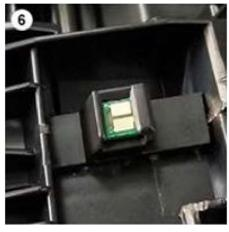
Insert the new **RevoSet** reset-chip into the chip holder
