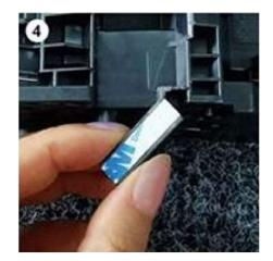
Apply a piece of double-sided tape to the back of the chip holder.
