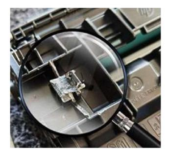
The **RevoSet** holder for reset chips on HP toner cartridges 59A/X replaces the original chip holder if it has been damaged during removal of the original chip.
